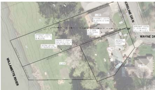
The existing storm drain and outfall provided drainage for the entire corner of the neighborhood.
